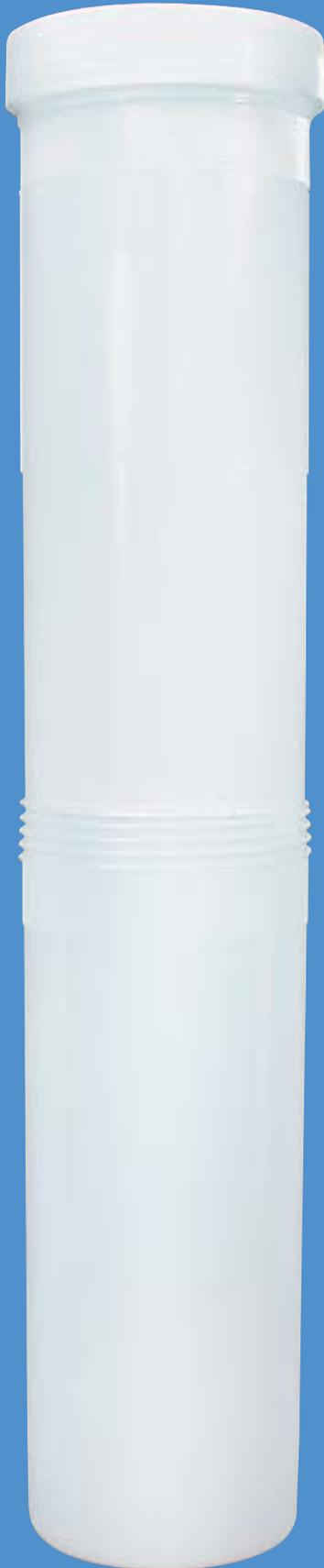
Large vessels are made by joining 2000 and 2200 ml jars using an infrared fusion process. The bottom is removed from the top jar and aligned with the threaded area of the lower jar. Infrared heat (1800°F) provides molten surfaces for fusion bonding. The bond is strong and pure – no extraneous materials added.
