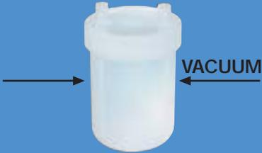
These containers do not deform at a vacuum of 29.1 inches of mercury. Containers registered a net loss of -0.1 inches after 60 minutes without additional pumping.
