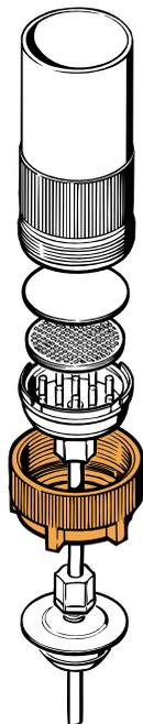
Exploded view of the 47 mm holder used with a side port suction flask. Shown with #007-6 stopper in TEFLON®, page 24.
