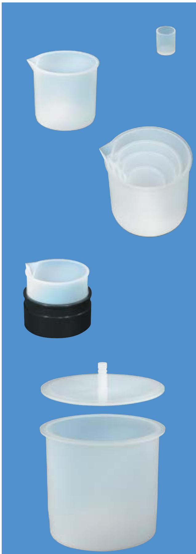
**BEAKERS:** Special features for microwave or hot plate. All beakers are molded with seamless solid bottoms. Bottoms are machined flat after molding for maximum contact with hot plates. The miniature (2 ml) beaker has straight sides. All other beakers have safe handling rims and pour spouts. Top surface of all beakers is flat. Next larger beaker could serve as cover. One beaker kit is suggested.
